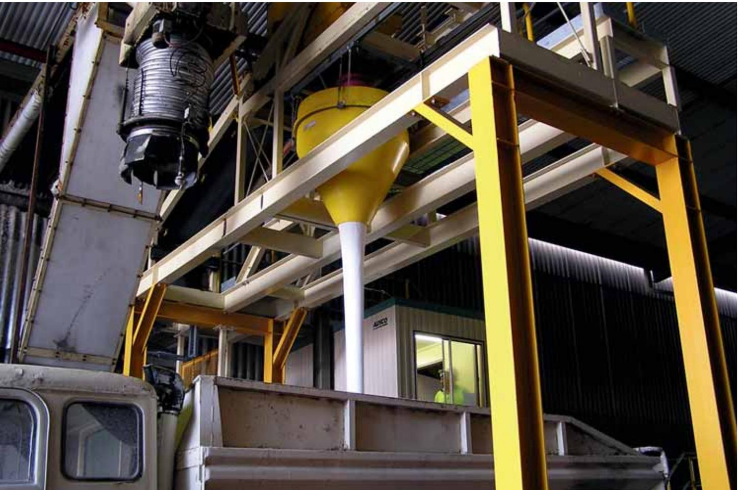
Fallout from bulk loading dry goods is now a thing of the past with the development of DSH Systems Ltd (dust suppression hopper) which fertilizer companies in New Zealand, Australia, North and South America and South Africa have embraced to control their dust and provide a cleaner and safer work environment.
