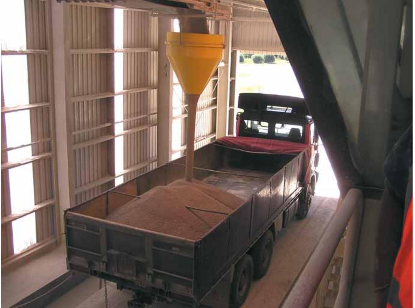
“We use the dust-suppression hopper on our load-out points; truck and rail and also the dress belt into store, a drop of about 14 metres.
