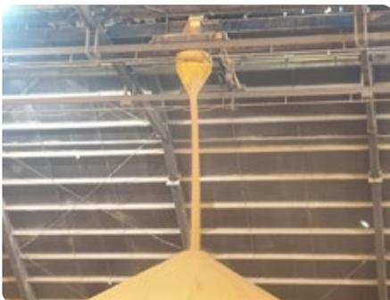
At the point of loading, the DSH system concentrates the discharge of bulk cargo into a solid column with minimal secondary dust. The hoppers require no electric power and have no internal moving parts.
