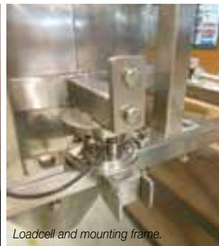
Loadcell and mounting frame.
